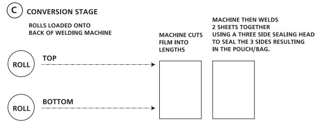
ROLLS ARE LOADED ONTO THE MACHINE TO MAKE SURE THE TWO LAYERS WHICH COME INTO CONTACT ARE THE FILM 5-LLDPE LAYER.
