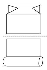
Tear off at the serrations. Bottom welded bag with side gussets to provide more volume.
