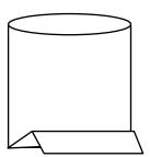
We put a crease in the fold in the bottom that effectively creates a flat bottom at the base of the bag.
