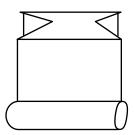
The box shape allows for a greater volume of product. We fold creases into the tubing as part of the manufacturing process.
