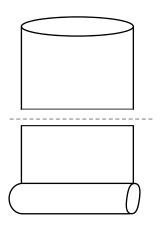
Tear off at the serrations. Bottom welded bag.
